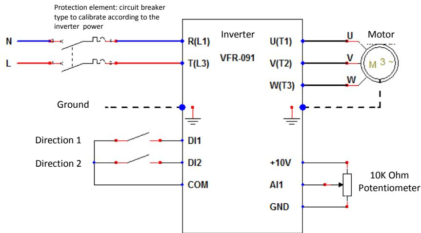
*Wiring example with a single phase inverter; also available in three phase*
