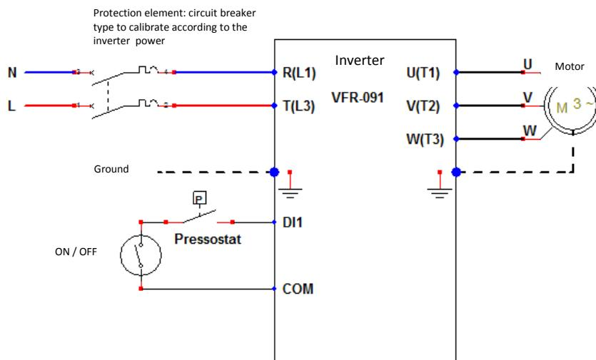
Wiring example with a single phase inverter; also available in three phase
