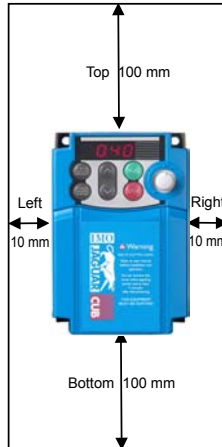
Figure 2.1 Mounting Direction and Required Clearances
