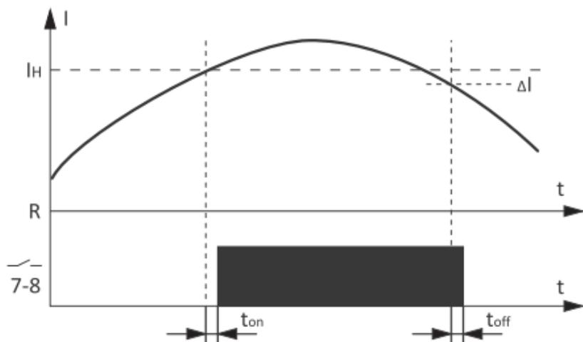
If the current in the measuring circuit exceeds the "Hi" setpoint, the relay contacts 7-8 will close and the contacts 9-10 open.
