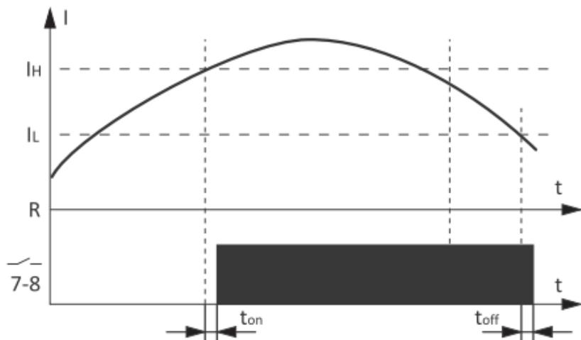
If the current in the measuring circuit exceeds the **Hi** setpoint, the relay contacts 7-8 will close and the contacts 9-10 open. The relay contacts in this function will only return to their original position if the current value is lower than **Lo**.
